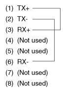
Figure F-2 LAN Loopback Connector
